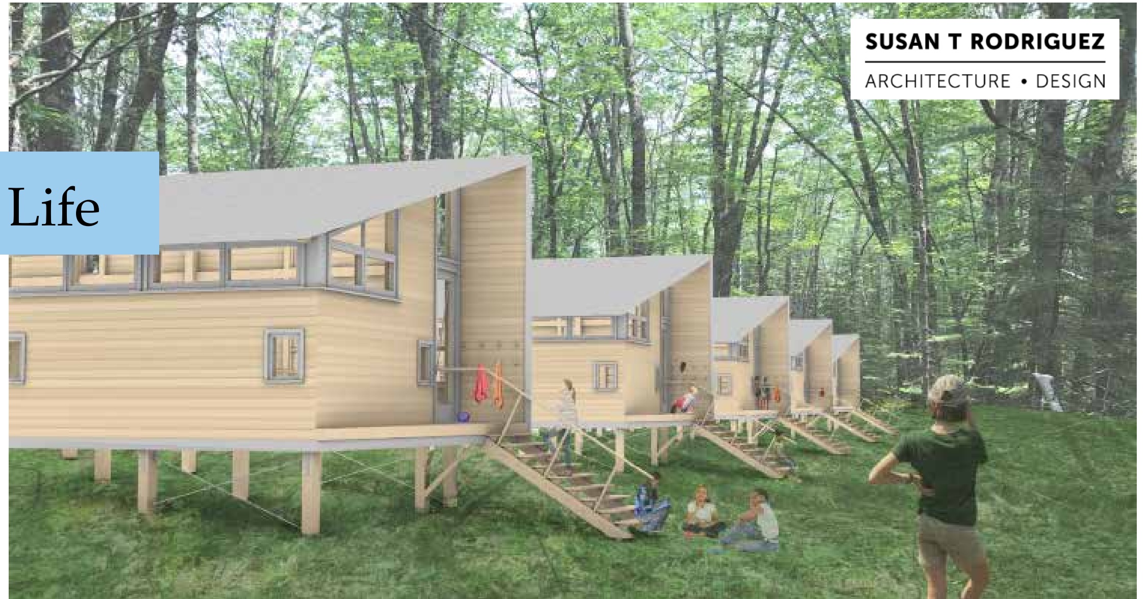
Above: A row of five cabins will provide housing for Camp Chewonki for Girls on the east side of Chewonki Neck. High ceilings and wraparound windows provide excellent ventilation and illumination inside. On the lower level, each bed has an operable shuttered window to let in the light--or keep out the commotion--as the occupant prefers. The post-and-beam cabins are sheathed in spruce with a natural finish that will blend into the forest backdrop over time.
