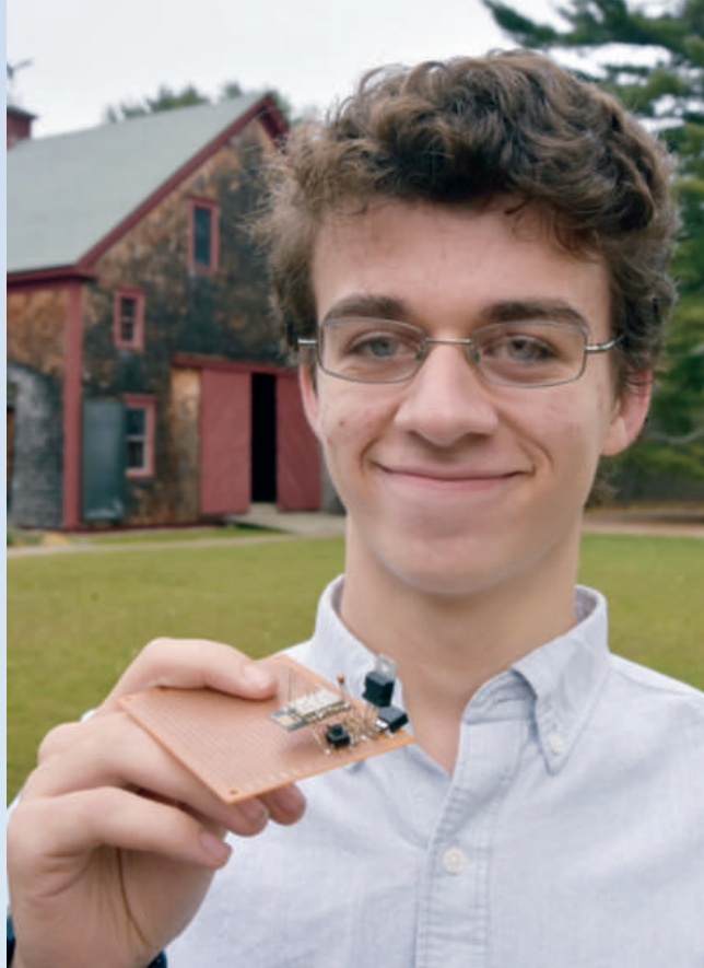
Noah Cowie (Sem. 55) holds a wireless thermistor he created as part of his Human Ecology Capstone. It will help monitor heat consumption in the Wallace Center.
